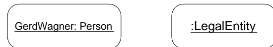
Figure 4: Two agents: the agent GerdWagner , as an instance of the agent type Person , and a prototypical instance of LegalEntity .
