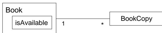
Figure 1: A library database includes two object types: Book and BookCopy . Books for which the status predicate isAvailable holds (determined by checking if there is at least one copy of that book available) form a subclass of Book .
