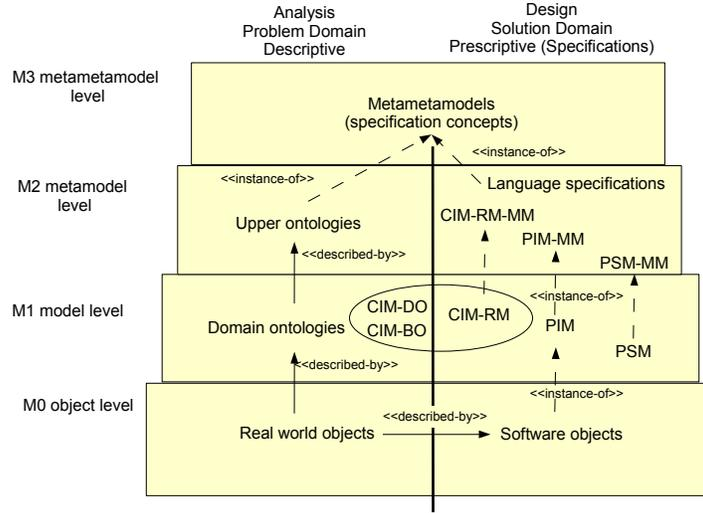
**Fig. 9.** A proposal for the role of ontologies in meta-pyramid of model-driven engineering and the MDA.
