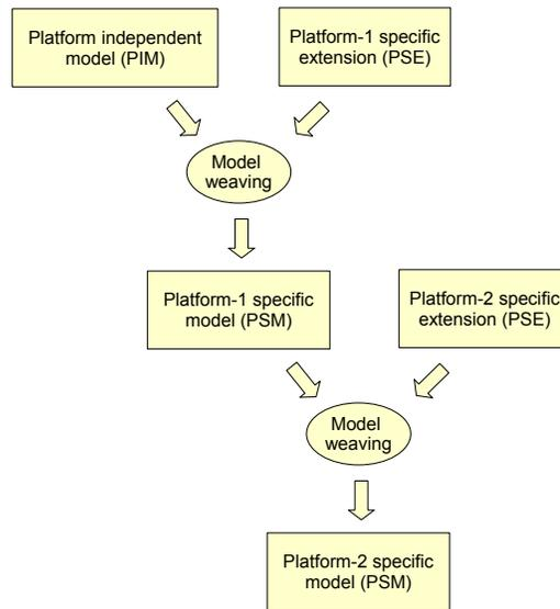
**Fig. 3.** The MDA pattern: weaving a platform-specific extension as an aspect into a PIM as a base.
